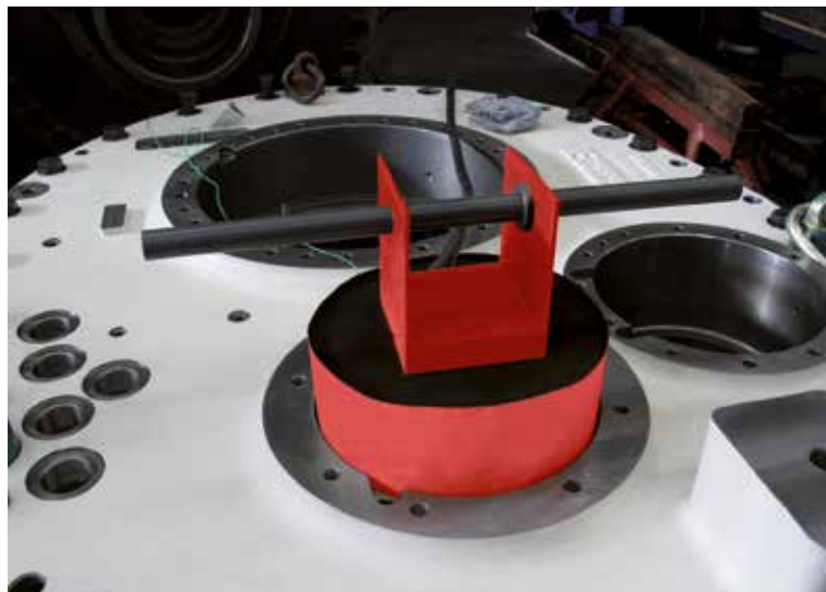
Heating bores in housings For mounting bearings and pins (including in frames and gearboxes).
